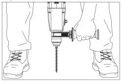
If the speed begins to drop off when drilling large or deep holes, pull the bit partially out of the hole while the tool is running to help clear dust. Do not use water to settle the dust since it will clog the bit flutes and tend to make the bit bind in the hole. If the bit should bind, a built-in, non-adjustable slip clutch prevents the bit from turning. If this occurs, stop the tool, free the bit and begin again.
